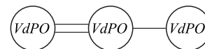
FIG. 1. The model of an open array of van der Pol's oscillators (VdPO).
